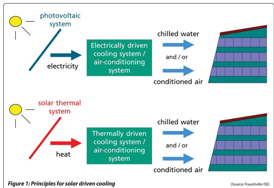
refrigeration systems using solar thermal energy as the main driving energy.
