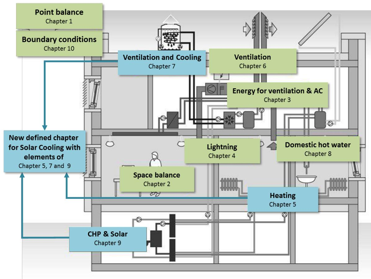
Figure 3: Elements of the DIN V 18599 that can be used for defining a separate chapter for Solar Cooling Systems (Source: DIN / JER)
