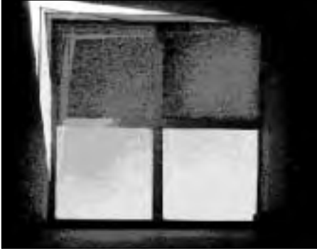
An electrochromic window developed by NREL in the United States.
