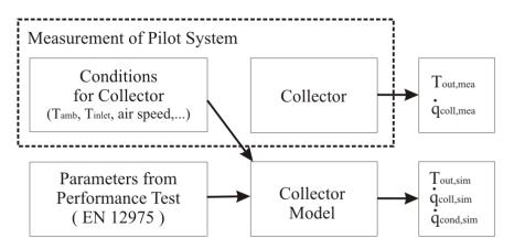
Fig. 2: Schematic procedure to determine the condensation gains in the monitored system from the measured data. The comparison of outlet temperature Tout and collector yield  $\dot{q}_{coll}$  indicates the accordance of simulation. The yield through condensation is determined within the simulation model.
