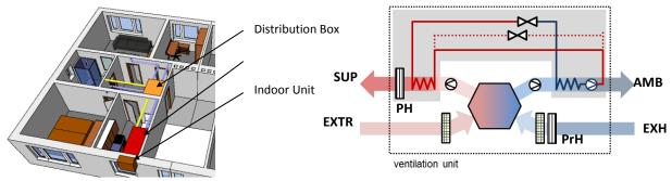
Fig. 2: 3D view of the flat with the supply air heat pump system (left) and scheme of the heat pump in combination with MVHR (right). "PH" and "PrH" represent the post-heater and the pre-heater, respectively Siegele 2018
