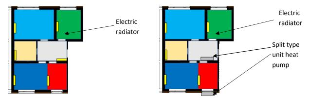
Fig. 8: 2D view of the flat with (left) electric radiators and (right) the HP split unit with recirculation of air in the corridor (Ochs et al. 2017). The indoor unit is installed in the corridor, while the outdoor unit can be integrated in the façade. All the rooms (except the corridor) are equipped with electric radiators
