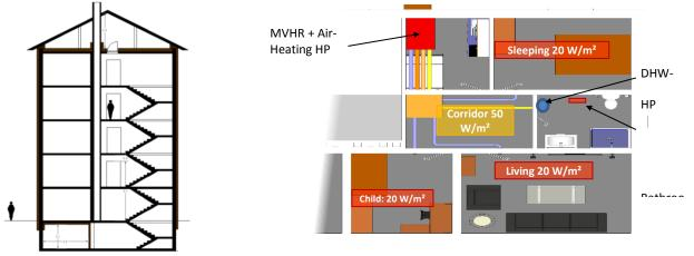
Fig. 1: (left) Typical MFH and (right) heat load (in W/m<sup>2</sup>) of the thermal zones with optional recirculation air heating in the corridor; Ventilation and HP in the kitchen and DHW HP in the corridor
