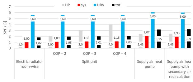
Fig. 11 Annual (heating season) SPFs of the heat pump ("HP"), heating system ("sys"), HRV and total HVAC ("tot"), according to equations (1)-(4)
