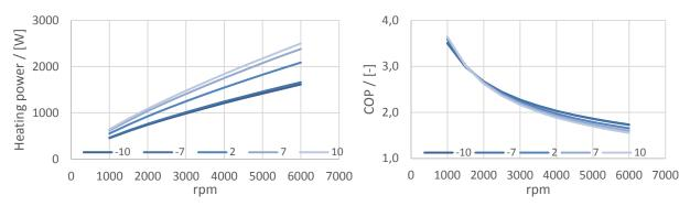
Fig. 6: Performance map of the thermal power of the heat pump (left) and the COP (right) depending on the rpm of compressor and ambient air temperature [°C] – Supply air heat pump system
