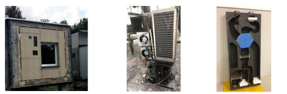
Fig. 5: Outside view of the outdoor unit integrated into the prefabricated timber frame façade in the Passys test cell (left), outdoor unit in the laboratory at the UIBK (center) and indoor unit
