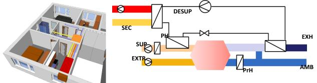
Fig. 3: 3D view of the flat with the supply air heat pump system with recirculation air in the corridor (left) and refrigerant cycle scheme (right). "PH" and "PrH" represent the post-heater and the pre-heater, respectively. "DESUP" indicates the de-superheater that is used to heat the recirculation air in the corridor, (Siegele 2018)
