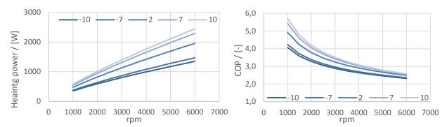
Fig. 7: Performance map of the total thermal power of the heat pump (left) and the COP (right) depending on the rpm of compressor and ambient air temperature [°C] – Supply air heat pump with secondary air recirculation system. Additional ambient air of 200 m3/h was used as source. The total heating power was split between the condenser (50%) for the supply air and the de-superheater (50%) for secondary air.
