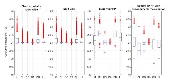
Fig. 10: Box plot of operative temperatures (hourly average) during the heating season for the four heating concepts
