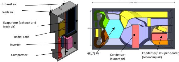
Fig. 4: 3D view of the outdoor unit with evaporator and compressor (left) and the indoor unit (right) with HRV/ERV, supply air condenser and secondary air condenser
