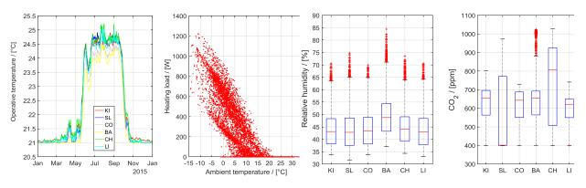
Fig. 9: Electric radiator room-wise system - daily average operative temperatures for each room of the flat (left) and hourly heating load versus ambient temperature (2nd from left); KI: Kitchen, SL: Sleeping Room, CO:
