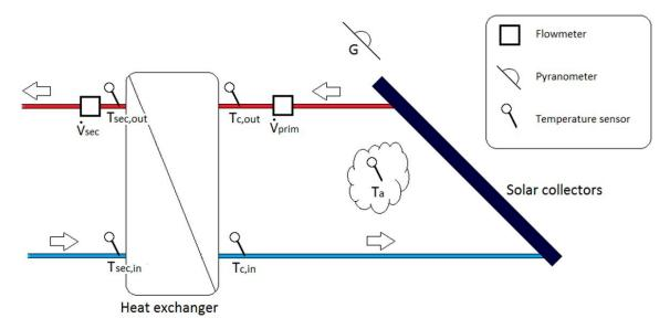
Fig. 2. Schematic drawing showing the measurement points.  $T_{c,out} = T_{prim,in}$  and  $T_{Cc,in} = T_{prim,out}$ . (Source: PlanEnergi)
