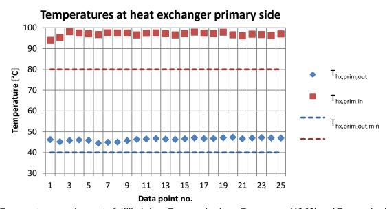
Fig.6. Temperature requirements fulfilled since T<sub>hx,prim,out</sub> is above T<sub>hx,prim,out,min</sub> (40 °C) and T<sub>hx,prim,in</sub> is above
