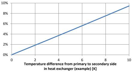
Figure 1. Example of the influence of the heat exchanger on the performance of the solar system. The higher the temperature difference across the heat exchanger ( $\Delta T$ ) the higher the temperature in the collector loop and the lower the collector performance. The influence of the heat exchanger depends on the heat loss coefficient of the solar collector: The higher the collector heat loss coefficient - the larger the influence of the heat exchanger. (Source: PlanEnergi)
