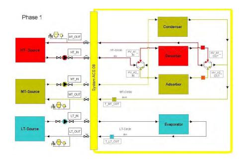
Figure 30: Main internal hydraulic components of the SorTech chiller and external connections. The figure presents the operation phase, of which the upper of the two sorption compartments is currently being desorbed by applying hot water and the lower sorption compartment is working as adsorber, thus taking up the vaporized refrigerant. The refrigerant circle, either fluid or vaporized, is not included into the figure. [Rupp, 2009]
