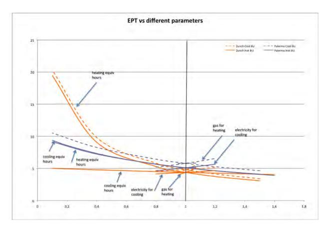
Figure 21: Relationship between  $E_{\mbox{\scriptsize PT}}$  and several parameters for Absorption Solar Cooling systems with hot and cold back-up
