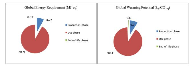
Figure 12: Percentage contribution of different phases of the plant life-cycle to GER and GWP for Zurich
