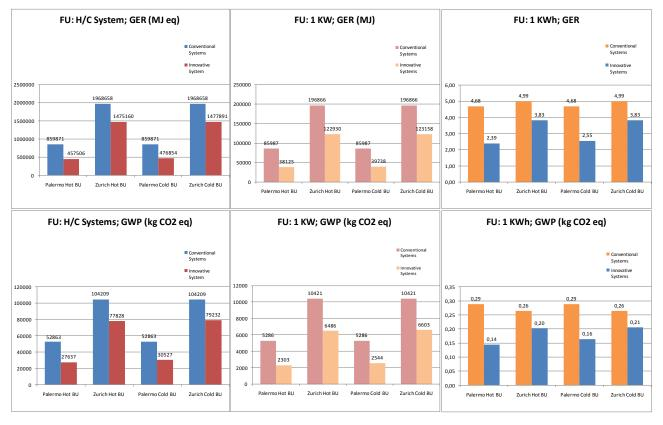
Figure 19: GER and GWP Absorption Solar Cooling systems with hot and cold back-up for different FUs and in comparison with conventional heating and cooling plants
