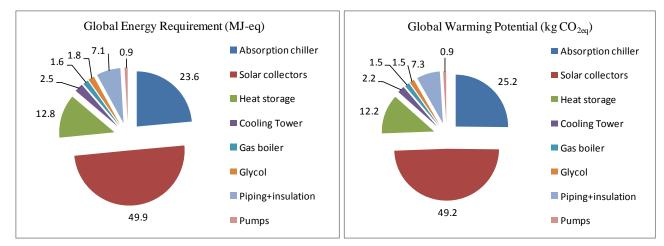
Figure 14: Production phase. Percentage contribution of different plant components to GER and GWP for Zurich
