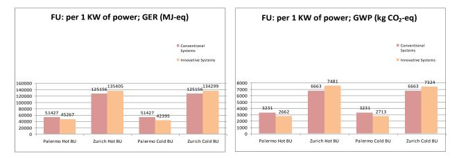
Figure 40: Comparison per 1kW of cooling power during 25 years of energy use in both climates and both back-up for GER and GWP
