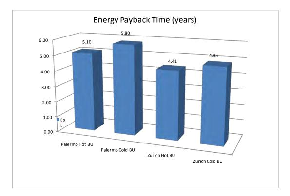
Figure 20: $E_{PT}$  for Absorption Solar Cooling systems with hot and cold back-up
