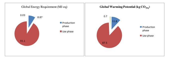
Figure 16: Percentage contribution of different phases of the plant life-cycle to GER and GWP for Zurich
