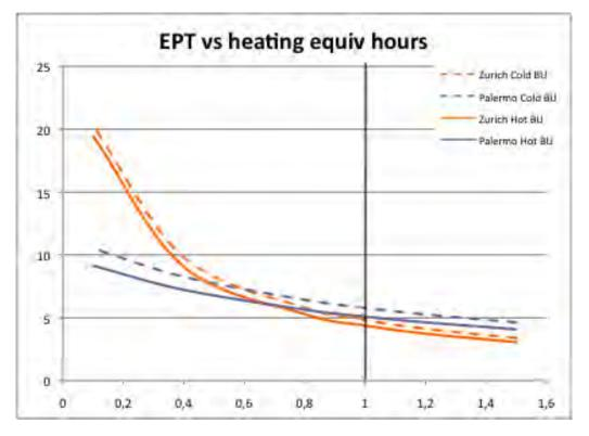
Figure 22: Relationship between  $E_{PT}$  and the number of equivalent hour of heating operation for Absorption Solar Cooling systems with hot and cold back-up
