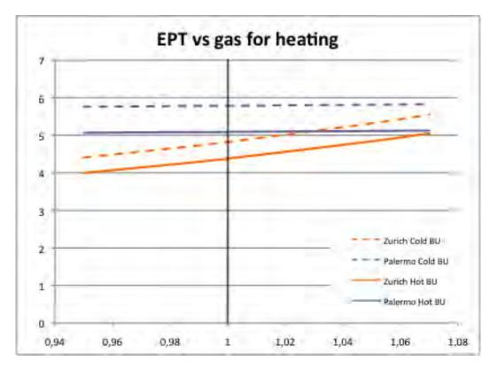
Figure 25: Relationship between  $E_{\text{PT}}$  and gas consumption for Absorption Solar Cooling systems with hot and cold back-up
