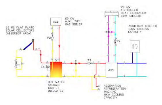
Figure 28: Schematic representation of the adsorption chiller plant
