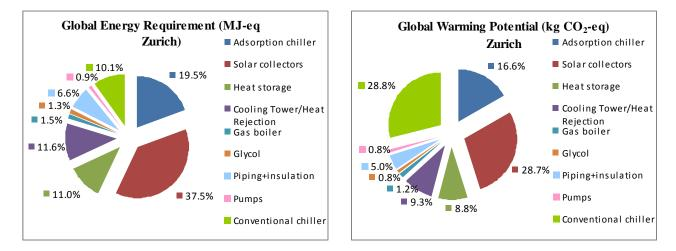
Figure 36: Production phase: Percentage contribution of different plant components to GER and GWP for Zurich
