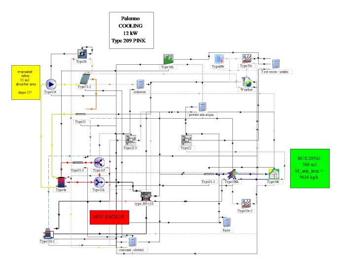
Figure 2: TRNSYS project for simulation of the absorption chiller plant with auxiliary boiler
