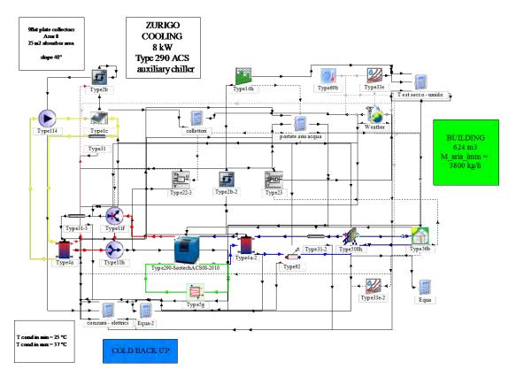
Figure 3: TRNSYS project for simulation of the adsorption chiller plant with cold back up
