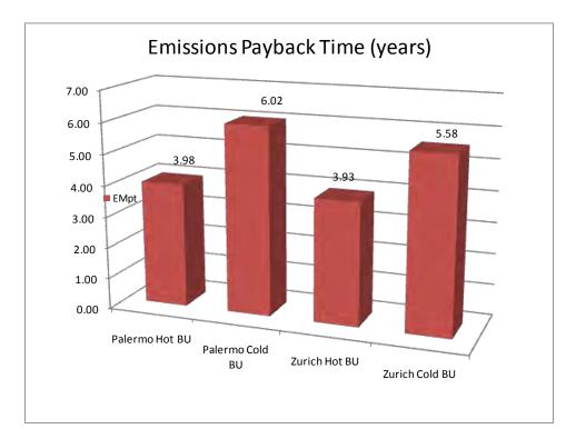
Figure 26: Emissions Payback Time for Absorption Solar Cooling systems with hot and cold back-up
