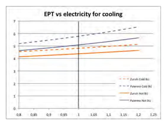
Figure 24: Relationship between  $E_{\text{PT}}$  and electricity consumption for cooling operation for Absorption Solar Cooling system with hot and cold back-up
