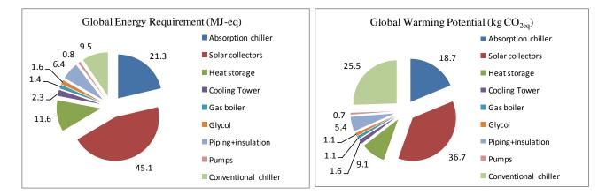
Figure 18: Production phase. Percentage contribution of different plant components to GER and GWP for Zurich
