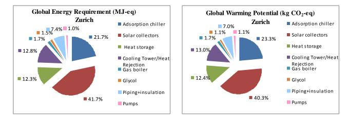
Figure 32: Production phase: Percentage contribution of different plant components to GER and GWP for Zurich
