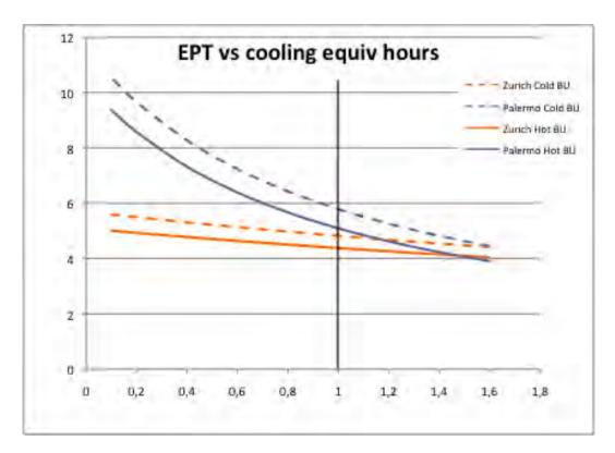
Figure 23: Relationship between  $E_{PT}$  and the number of equivalent hour of cooling operation for Absorption Solar Cooling systems with hot and cold back-up
