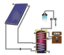
Figure 50: Hydraulic scheme of the domestic hot water pumped reference system for single-family houses
