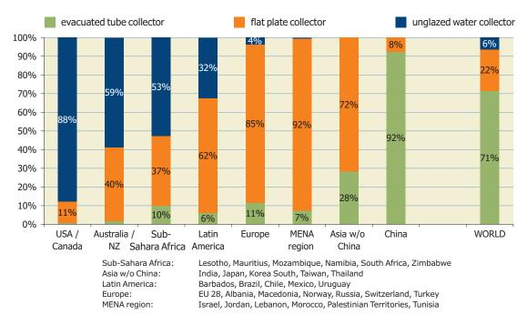
Figure 34: Distribution by type of solar thermal collector for the total installed water collector capacity in operation by the end of 2014
