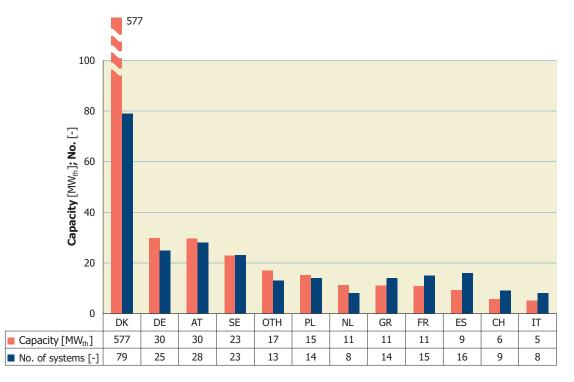
Figure 41: Solar district heating and cooling in Europe – capacities installed and No. of systems in 2015 (Data source: Jan-Olof Dalenbäck – Chalmers University of Technology, SE)
