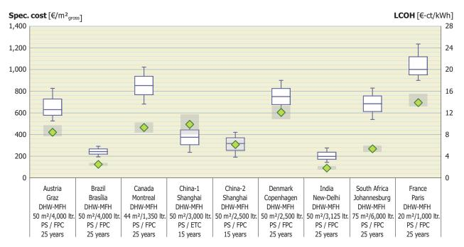
Figure 46: Specific Investment costs and levelized costs of solar thermal generated heat for large *pumped* domestic hot water systems
