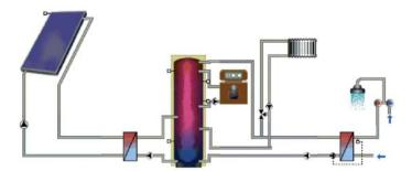
Figure 53: Hydraulic scheme of the solar-combi reference system for single and multifamily houses
