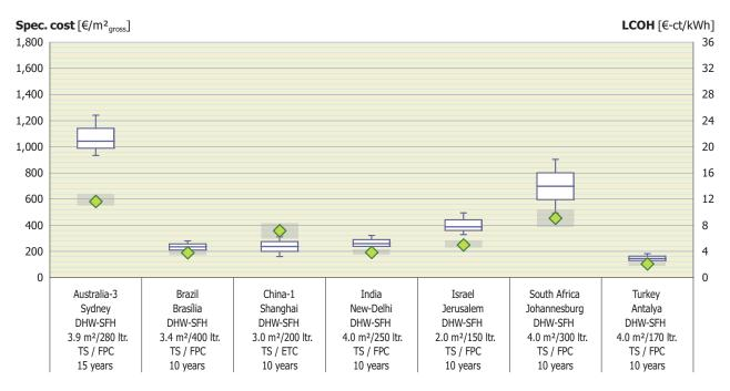
Figure 45: Specific Investment costs and levelized costs of solar thermal generated heat for small thermosiphon domestic hot water systems
