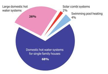
**Figure 30:** Share of energy savings and CO<sub>2</sub> reduction by type of application of glazed and unglazed water collectors in operation in 2014
