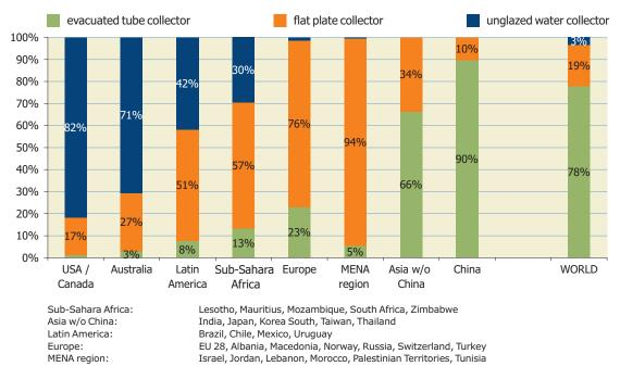
Figure 35: Distribution by type of solar thermal collector for the new installed water collector capacity in 2014
