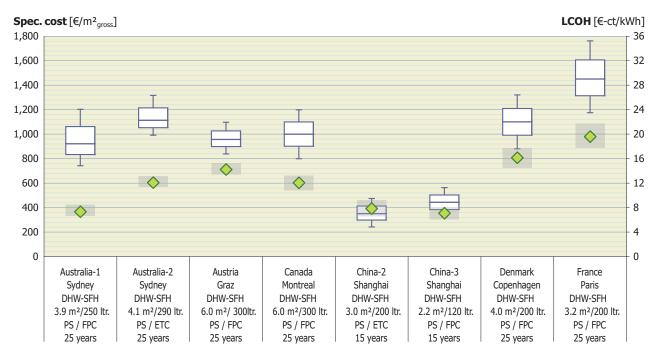
corresponding **levelized costs of solar thermal generated heat (LCOH)** in €-ct/kWh<sup>23</sup> are shown as grey bars (green diamond equal the average value).
