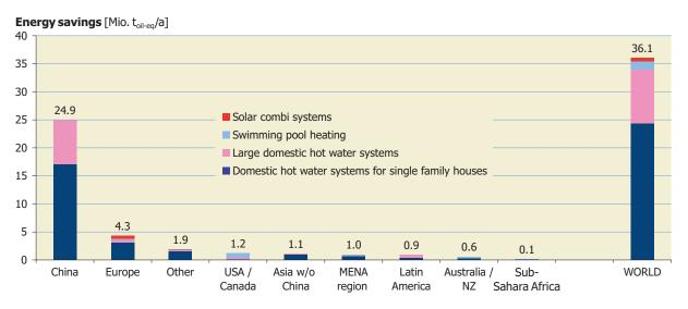
Figure 32: Annual energy savings in oil equivalent by unglazed and glazed water collectors in operation in 2014
