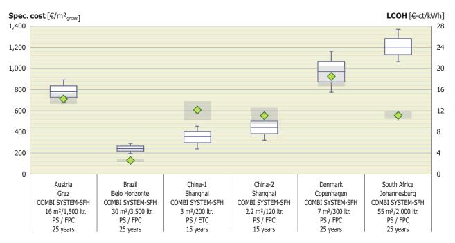
Figure 47: Specific Investment costs and levelized costs of solar thermal generated heat for small combined hot water and space heating systems
