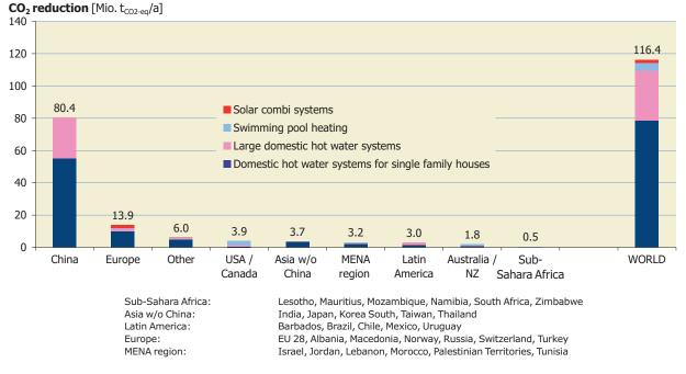
Figure 33: Contribution to CO<sub>2</sub> reduction by unglazed and glazed water collectors in operation in 2014
