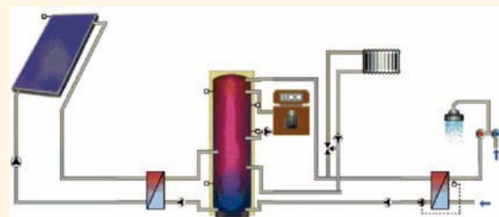
Hydraulic scheme of the solar-combi reference system for single and multifamily houses
