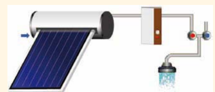
Hydraulic scheme of the domestic hot water thermosiphon reference system for single-family houses
