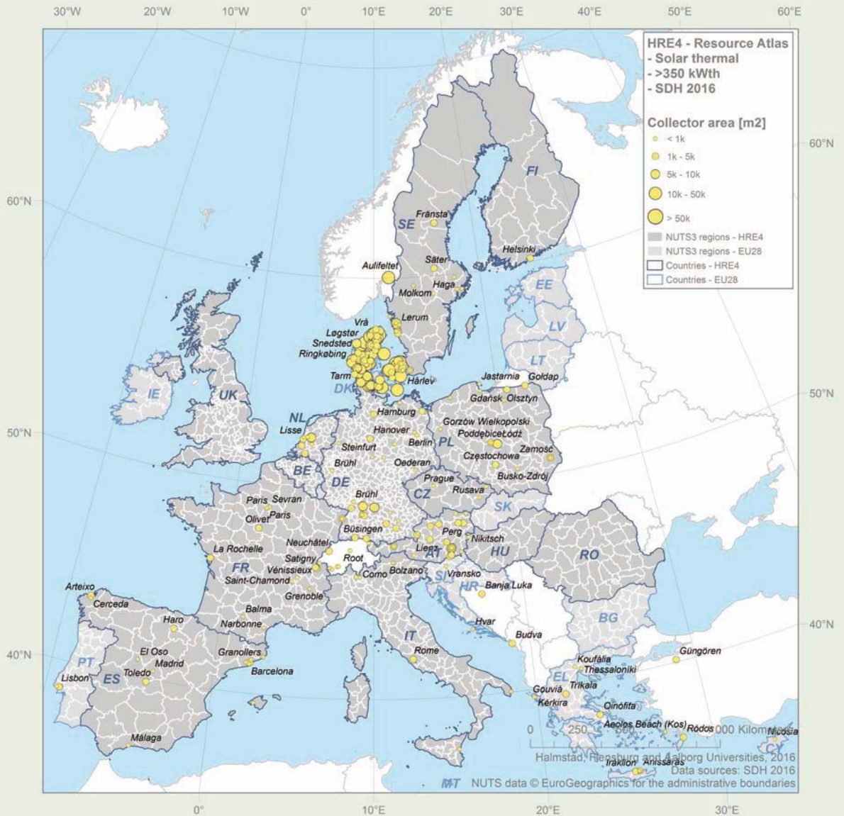
Figure 7: Solar district heating systems >500 m 2 (350 kW th ) in Europe. (Source: Heat Roadmap Europe)
