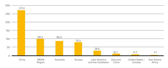
Figure 30: Total capacity of glazed flat plate and evacuated tube collectors in operation by economic region and in  $kW_{\rm th}$  per 1,000 inhabitants in 2021
