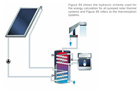
Figure 54: Hydraulic scheme of the domestic hot water pumped reference system for single-family houses
