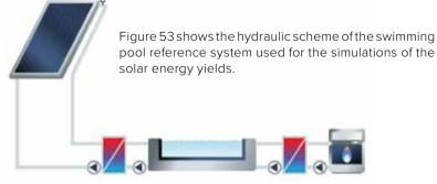
Figure 53: Hydraulic scheme of the swimming pool reference system
