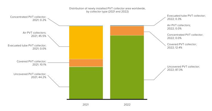
Figure 18: Distribution of newly installed PVT collector area worldwide by collector type in 2021 (left) 2022 (right) Source: AEE INTEC
