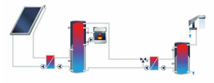
Figure 56: Hydraulic scheme of the domestic hot water pumped reference system for multi-family houses
