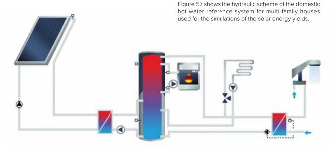
Figure 57: Hydraulic scheme of the solar-combi reference system for single and multi-family houses
