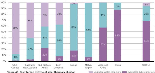
Figure 48: Distribution by type of solar thermal collector for the total installed water collector capacity in operation by the end of 2021
