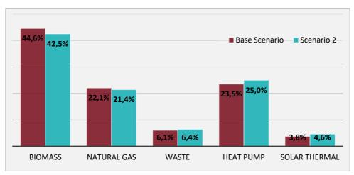
Figure 3: Sensitivity analysis of district heating generation in Austria (base scenario vs scenario with 20% higher price for gas and biomass)
