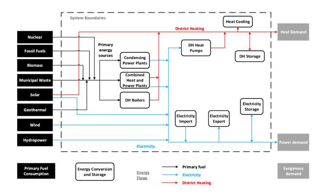
Figure 1: Core structure of Balmorel model [3]
