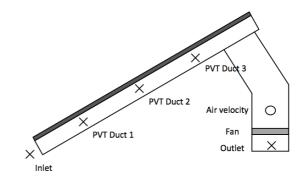
Figure 21 Schematic of thermocouple and air velocity sensor location
