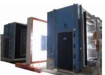
Figure 1 The image on the left shows a modular specimen of the prototype that has been conceived, developed and tested in the EURAC laboratory, in the calorimeter which is shown on the right.
