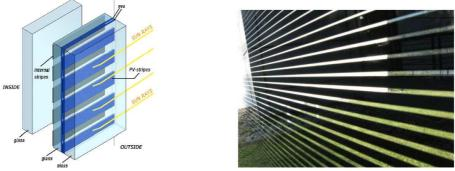
Figure 9 Left: schematic view of the new transparent, angle-selective façade. The stripes (represented in blue) can be produced with photovoltaic technology. On the right: a detailed view of the first prototype with black ceramic frit stripes.
