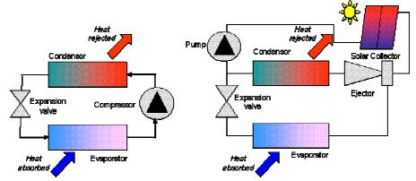
Figure 17 Solar driven ejector heat pump compared to a conventional electric heat pump.
