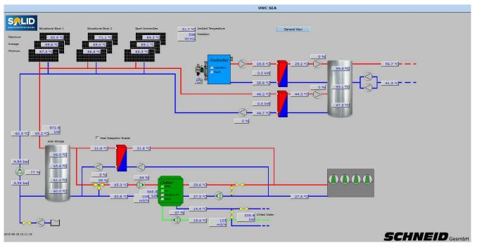
Figure 17: Monitoring scheme of the solar cooling system at the UWC (Source: SOLID)
