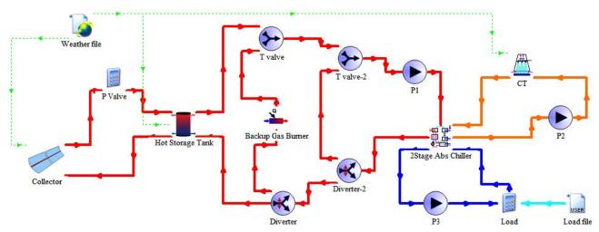
Figure 30: TRNSYS schematic of simulated solar cooling system with double-effect absorption chiller (Source: CSIRO)
