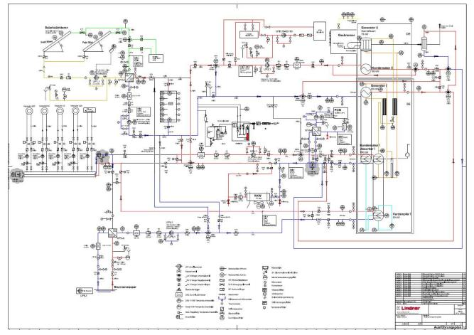
Figure 10: Hydraulic scheme of the solar cooling system (Source: ZAE Bayern)
