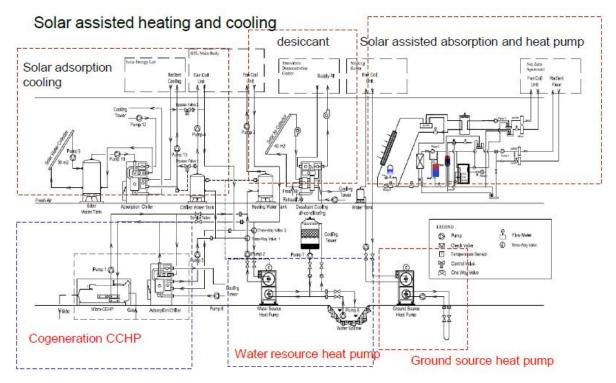
Figure 26: Scheme of GEL solar cooling and heating system (Source: SJTU)
