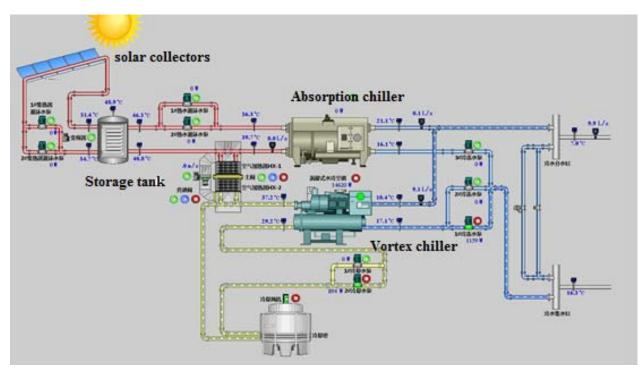
Figure 21: Scheme of the absorption chiller system with the vortex chiller (Source: SJTU)
