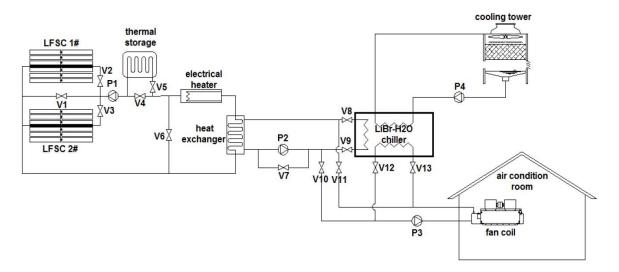
Figure 23: Schematic of the solar energy and heat storage system (Source: SJTU)
