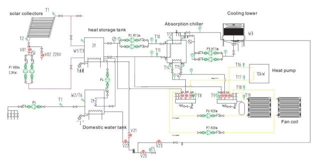
Figure 19: Scheme of the solar cooling system at the Linuo office building (Source: SJTU)
