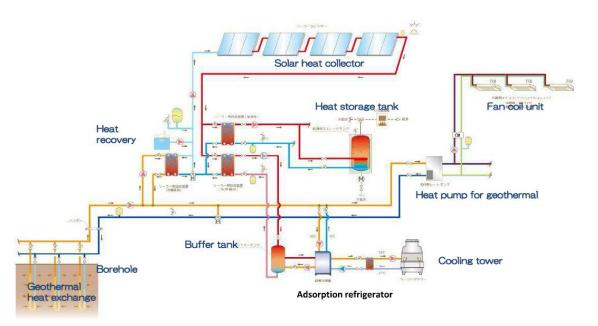
Figure 29: System flow of the cooling system (Source: Osaka Technocrat Ltd.)
