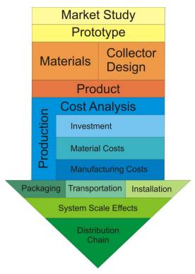
Figure 1: Schematic of the different steps of the cost calculation. At the end of each block the product has to pass the cost analysis. From top to bottom more detailed information about the value chain of the product is needed.
