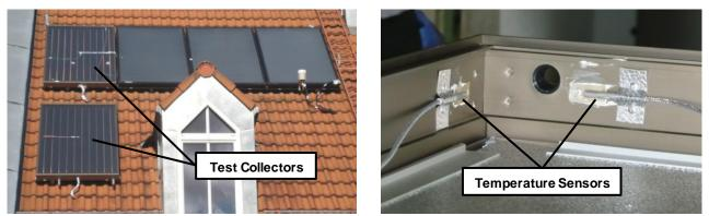
Figure 1: Field-testing of collectors (left) and exemplary temperature measurement equipment at a collector casing (right; Reiter et al. 2012)
