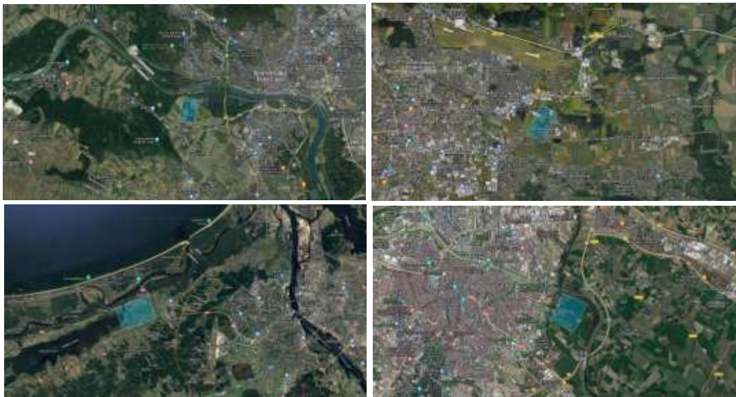
Figure 8 Illustration on the space demand of a solar thermal plant to satisfy 20% of the heat demand for Bratislava (1 171 280 m 2 area, 229 491 MWh/a), Klagenfurt (474 012 m 2 area, 109 205 MWh/a), Riga (6 741 504 m 2 area, 967 116 MWh/a) and Zaragoza (755 392 m 2 area, 287 793 MWh/a), from https://solardistrictheating.eu/ (currently restricted website), based on Google Maps and on an analysis done by Absolicon
