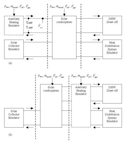
Figure 1: Two possible layouts of the test facility for solar combisystems.
