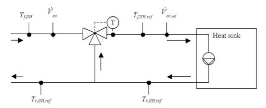
Figure 3: The Heat Distribution System Emulator.
