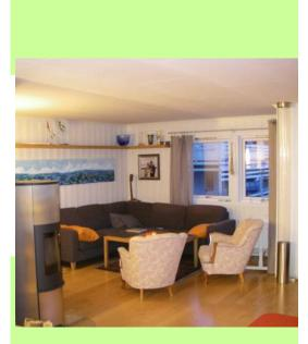
Living room after renovation. The transparent ventilation duct to the right provides fresh air to the office and one of the bedrooms in the base floor. A 5W LED lamp is installed within.
